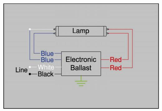
Notes: Applicable for 120V magnetic T12 to either T8 or T12 electronic fixtures. Always disconnect power to lighting fixture prior to servicing the fixture
